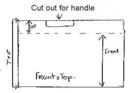
and adjust if needed. To make the flap to go under your handle measure the internal dimensions of your handle and make the flap so that it overlaps the front enough to be fastened down by the method of choice.
